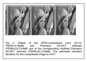
Once this global estimate is produced, it is used as reference estimate for an empirical Wiener filter in SA-DCT domain. Following the same adaptive averaging procedure as for hard-thresholding, we arrive to the final Anisotropic LPA-ICIdriven SA-DCT estimate. This procedure is called "*Pointwise SA-DCT*".
