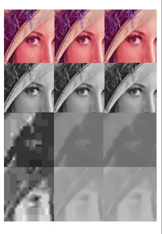
Fragments of the JPEG-compressed (Q=20, Fig. 3. PSNR=29.83dB), and restored Lena image using Pointwise SA-DCT (PSNR=30.9985dB) and Modified Pointwise SA-DCT (PSNR=30.9994dB). Top to bottom row: RGB color, luminance Y, and chrominance U and V channels.
